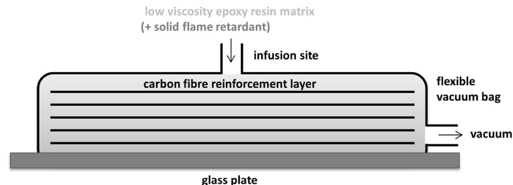
Fig. 3. Composite processing methods.
